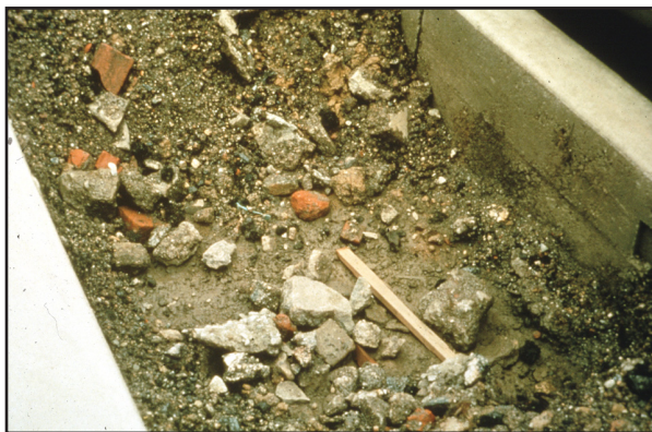
Fig. 59: Construction debris in soils can modify pH. NO construction debris should be dumped in planters.
