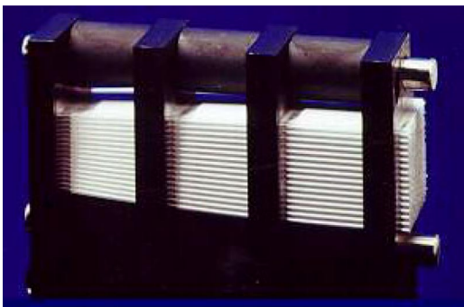
FIG. 2. Multifiber collimating lens with 20 \times 20 mm output, 8.07 \times 8.07 mm input, focal length (optimal distance to source) of 250 mm, length 127 mm, and transmission efficiency of 37% at 17.5 keV.
