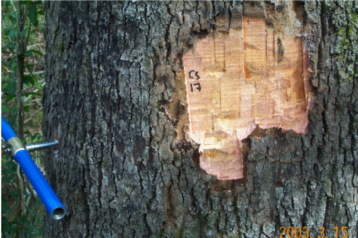
Figure 1: Tree boring (left) and bark sampling from a tree in Crystal Springs, MS, March 15, 2003.
