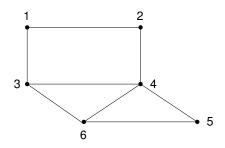
It is known that the local function associated with each of the nodes 1 through 4 is the 1-threshold function. It is also known that the local functions associated with nodes 5 and 6 are threshold functions; however, we *don't know* the corresponding threshold values.
