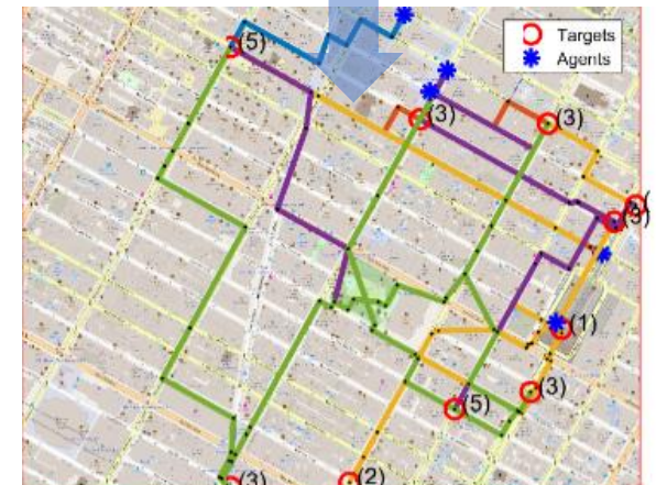
(f) Iter 5: Remove T_1 from A_3 's path, A_1 -costliest agent with all cardinality fulfilled
