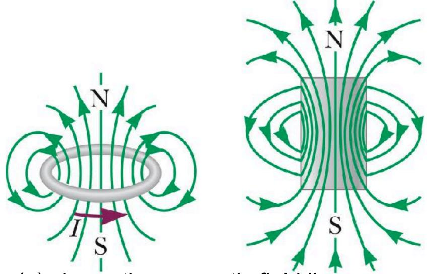
Figure (a) shows the magnetic field lines surrounding a current loop.
