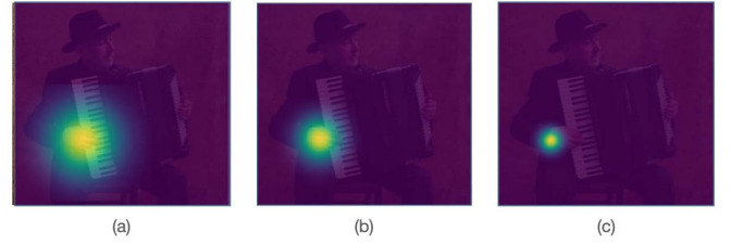
Fig. 5: Multi-scale supervision (MSS) can provide keypoint refinement analogous to the attention mechanism in resolution pyramid search. (a) to (c) are the 8x, 4x, 2x scales keypoint heatmaps respectively. The progression from (a) to (c) shows the refinement of keypoint heatmaps during the deconv up-sampling, where the location of the thorax keypoint is refined with increasing accuracy and more concentrated heatmap.
