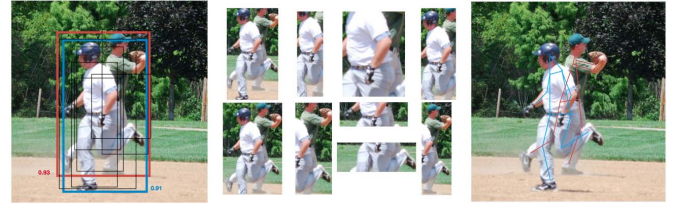
Fig. 1: Difficulties in top-down person detection and pose estimation, where a large number of bounding boxes including mostly redundant ones (in black color) co-exist around valid proposals (red and blue). IoU based non-max-suppression (NMS) in this case tends to keep only one (e.g. the red) proposal box after NMS, as the blue and red boxes (each for a person under heavy occlusion) are with high overlap. To correctly extract the poses of both individuals, existing top-down methods rely on lowering the NMS threshold to retain more-than-sufficient detection boxes to avoid possible miss-detection. Costly pose estimation must carry out on these redundant proposals which results in high computational cost.
