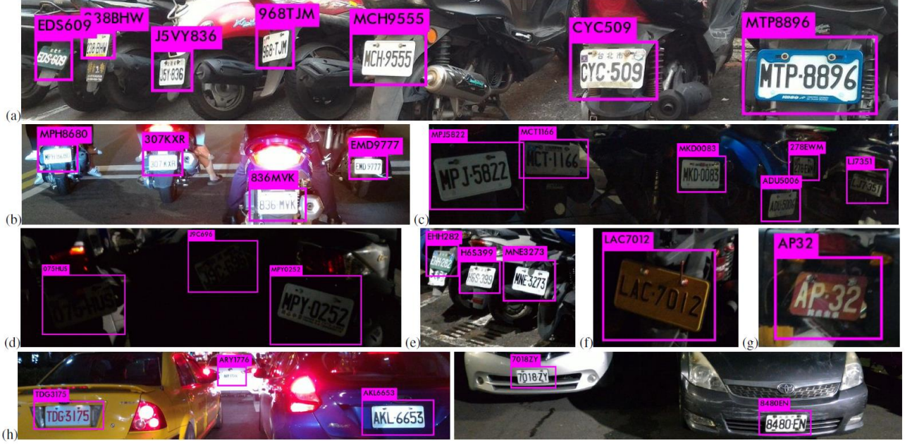
Fig. 3 Visual results of scooter ALPR in (a) day time, (b) strong reflectance/over-exposure, (c) night time, (d) dark lighting condition, (e) green LP, (f) yellow LP, (g) red LP for heavy motorcycles. (h) Our method can be used to detect car LPs as well.
