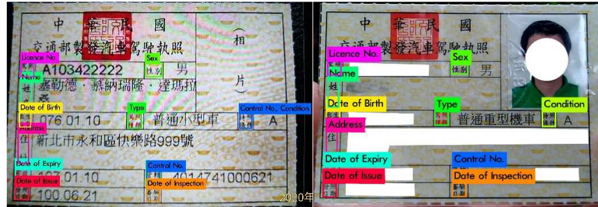
Fig. 3. Example of field detected result for viewing from an up-right angle.
