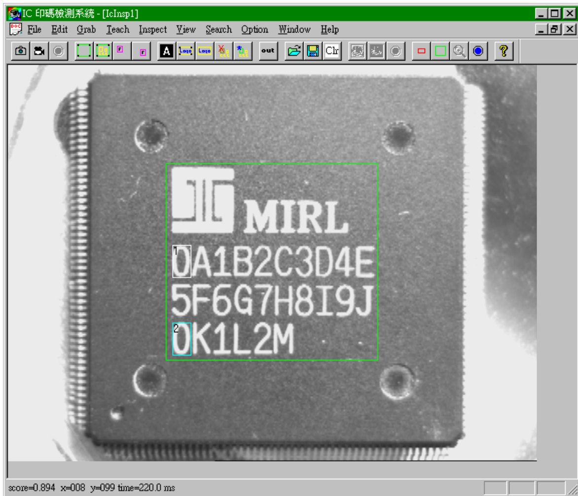
Figure 3.17: Two targets are successfully searched in an over-lighted image.
