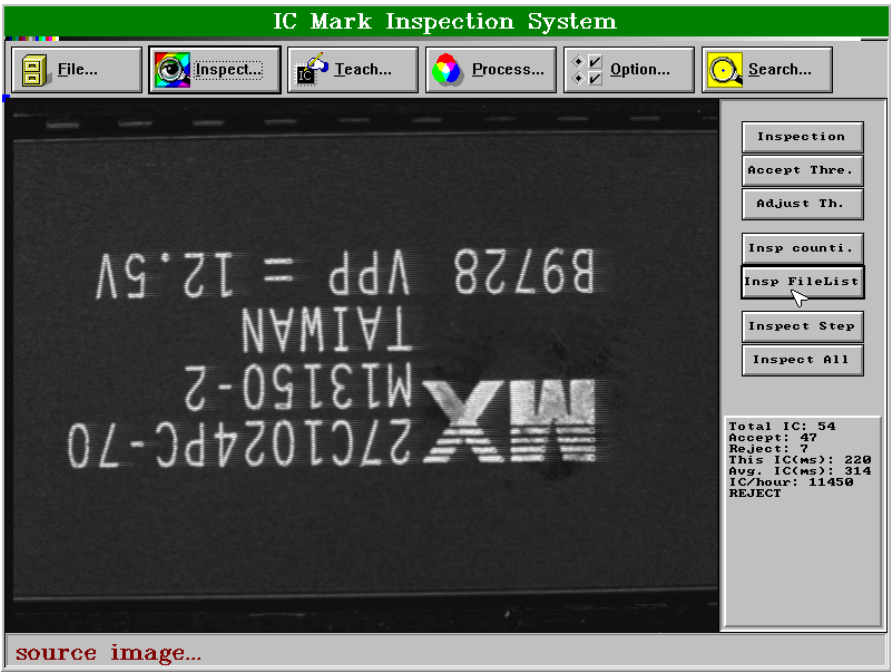
Figure 4.13: Test image of defective IC.
