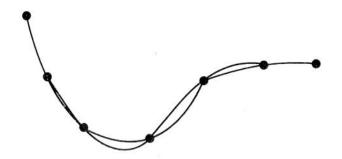
A linear blending function is then used to combine the sets of curves into a single curve through all the data points. This blending function has the value one at the middle of each quadratic and zero at the ends. The resulting curve is smooth, and will not exhibit waviness, however many points are to be interpolated.
