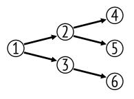
DAG, showing that task 1 must complete before tasks 2 and 3 can be started, etc.
