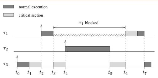
A priority inversion is said to occur in the interval  $[t_3, t_6]$ , since the highest-priority task  $\tau_1$  waits for the execution of lower- priority tasks  $(\tau_2 \text{ and } \tau_3)$ .
