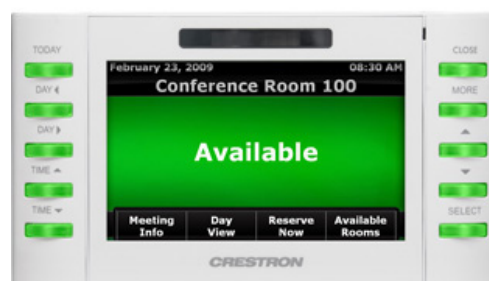
FIGURE 01.16 FIGURE 09.10 Sample point of use room scheduler panel that should be mounted outside classrooms and group study rooms of 24 stations or less to facilitate on-demand scheduling. The display clearly indicates who controls the room for a given time period.
