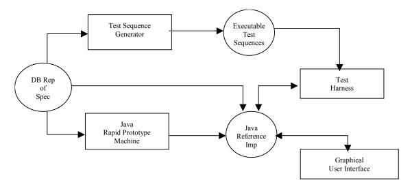
**Figure 7: Testing Tool Architecture**
