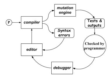
Figure 3: Integrating Mutation into an IDE
