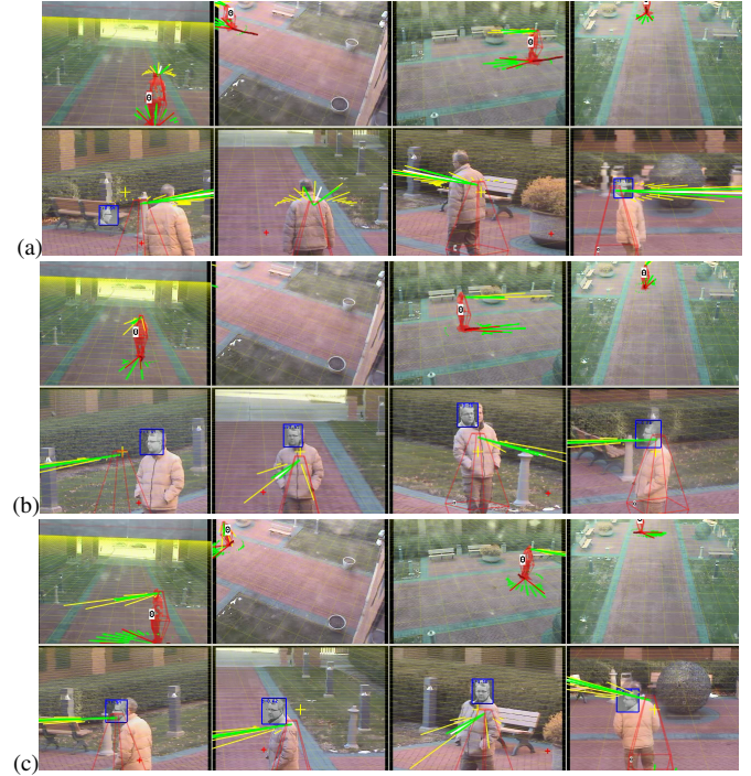
Figure 3. Pose and gaze estimation with face detections from PTZ cameras: (a) forward and (b) backward motion, (c) sideways glance with large difference between body pose and gaze. Overall tracking improves significantly when compared to Fig. 2.
