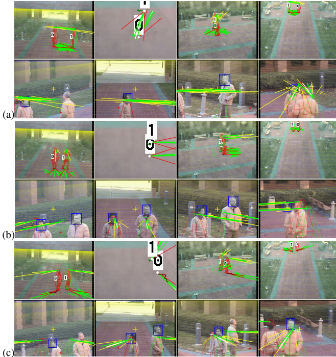
Figure 4. Pose and gaze estimation of two people (a) facing each other, (b) standing next to each other, and (c) facing in opposite directions. The top second view in each case depicts an artificial top-down re-rendering, which provides a better visualization of the relative pose and gaze.
