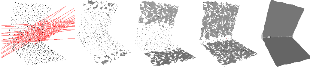
Fig. 12. Steps in reconstructing a “corner shape” from 800 sample points which illustrate how our method favors meshing triangles in the region distant to the corner prior to meshing sharp features, where difficult decisions (due to under-sampling) have to be made. From Left to Right: the full \mathcal{MS} (in red, with unbounded elements not shown); reconstructing the first 10%, 50%, and 90% of candidate triangles; final surface reconstruction result.
