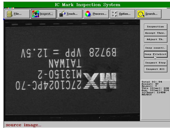
Figure 14: The defective IC print mark with partial bad contrast.
