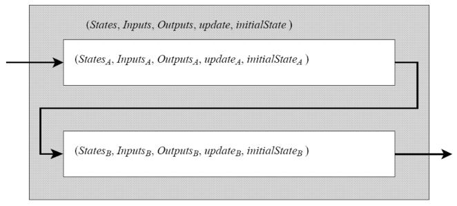
Synchronous composition: the machines react simultaneously and instantaneously, despite the apparent causal relationship!
