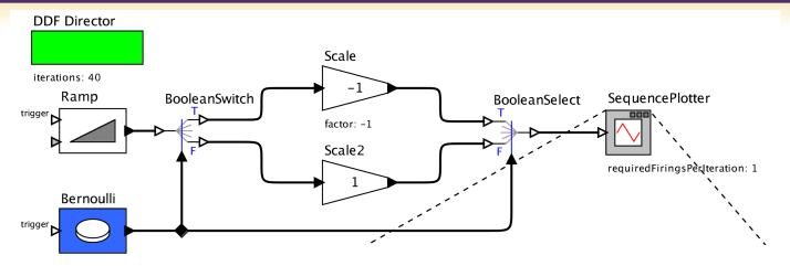
When Bernoulli produces true, the output of the Ramp actor is multiplied by -1
