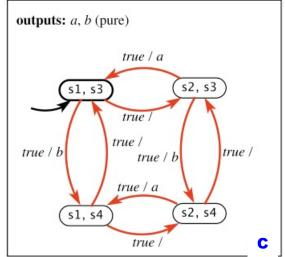
Asynchronous composition using <u>interleaving</u> semantics
