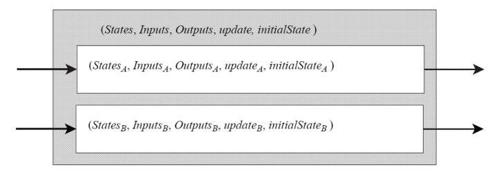
Synchronous composition: the machines react simultaneously and instantaneously.
