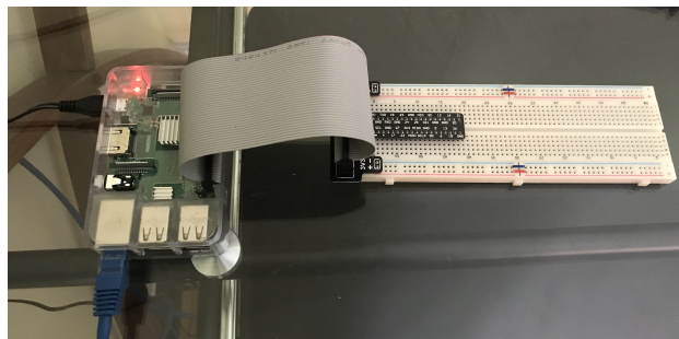
Figure 2.1: GPIO to Breadboard Interface Board and Ribbon Cable.
