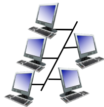
shared wire (e.g., cabled Ethernet)
