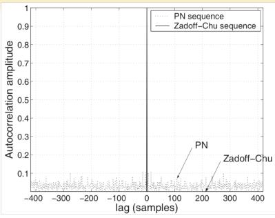
The ZC periodic autocorrelation is exactly zero for  $\sigma \neq 0$  and it is nonzero for  $\sigma = 0$
