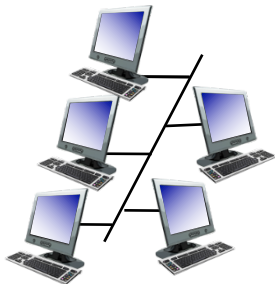
shared wire (e.g., cabled Ethernet)
